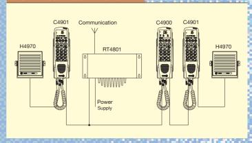
The SAILOR VHF RT4801 includes in a basic configuration a transceiver unit and a handset control unit. The units are connected by means of the SPARC-bus interface. This advanced balanced data and AF interface can be used to interconnect multiple control units as well as exterior computer based control/programming options. The maximum distance between transceiver unit and handset control unit may be up to 40m in 12VDC installations, in 24 VDC installations up to 80m.
