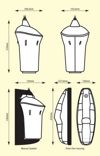
The SAILOR 406MHz Satellite EPIRB is a satellite distress beacon designed to operate in conjunction with the Cospas-Sarsat international satellite search and rescue system. This system locates beacons transmitting on the 406MHz frequency to within 5km (3nm). Once Search And Rescue (SAR) units are at the distress scene the beacon's 121.5MHz homing transmitter and it's high intensity xenon strobe light aid final location even in poor visibility.
